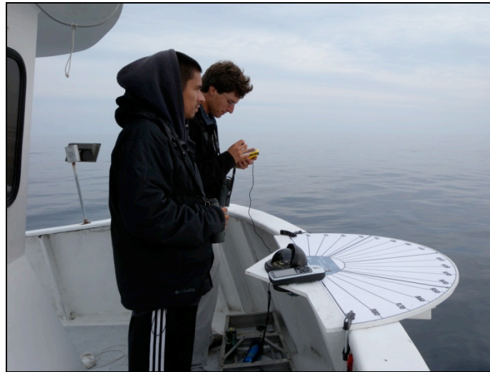
Fig. 25. Ship-based line transect surveys were conducted on a large vessel (>27.5 m), with one primary observer and one observer/recorder. Angle to birds was measured using a large protractor mounted to bridge railing. Note recorder (K. Winiarski) taking observations on a PDA, while primary observer (B. Harris) is actively searching for birds with both naked eye and binoculars.
